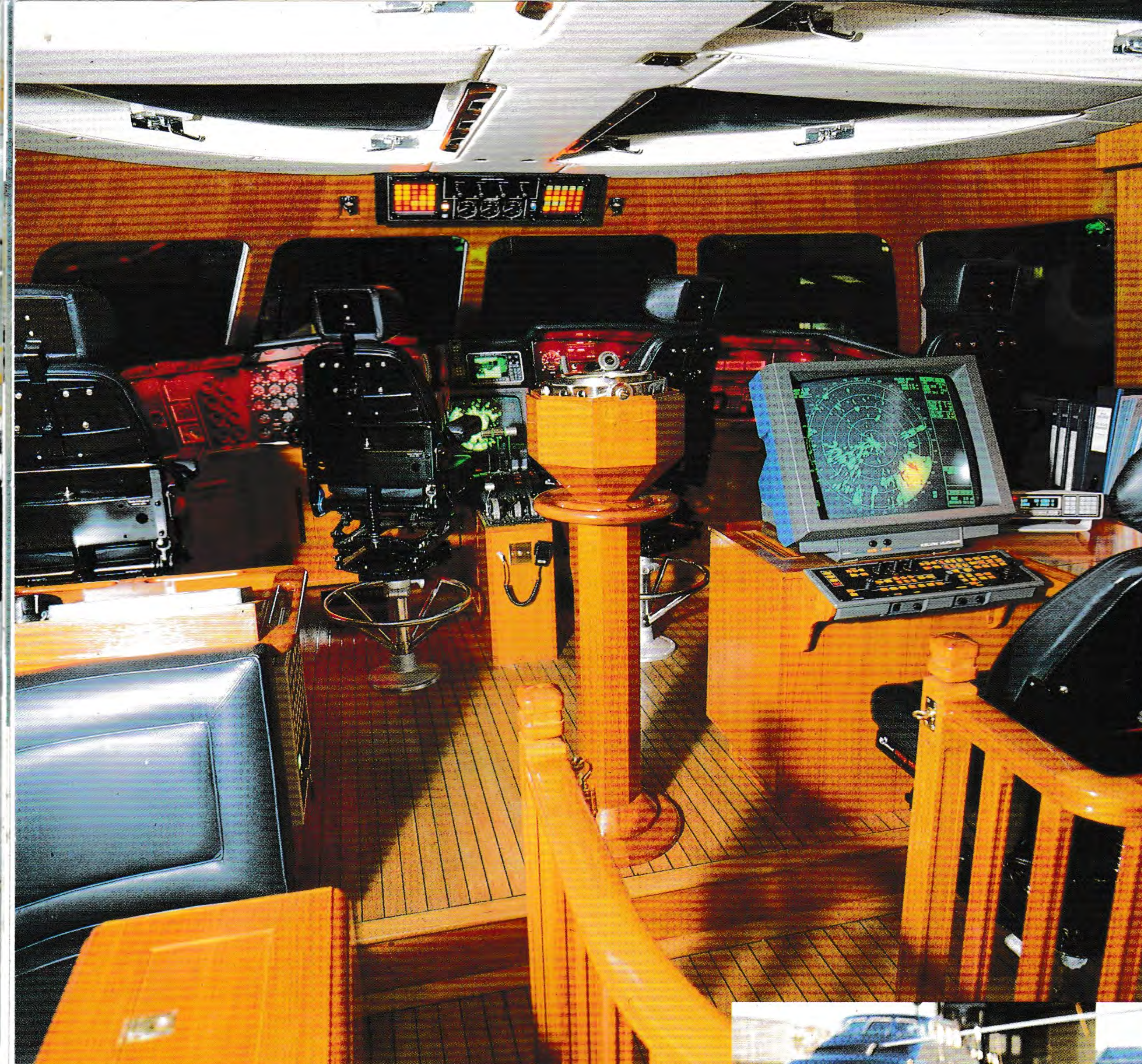
The bridge of Brave Challenger, added to the ship during her restoration, was completed to aircraft standard. To the right, the navigator's position features a large screen ARPA anti-collision radar and a state-of-the-art satellite navigation system. The central teak pedestal houses the ship's traditional gyro-compass.
